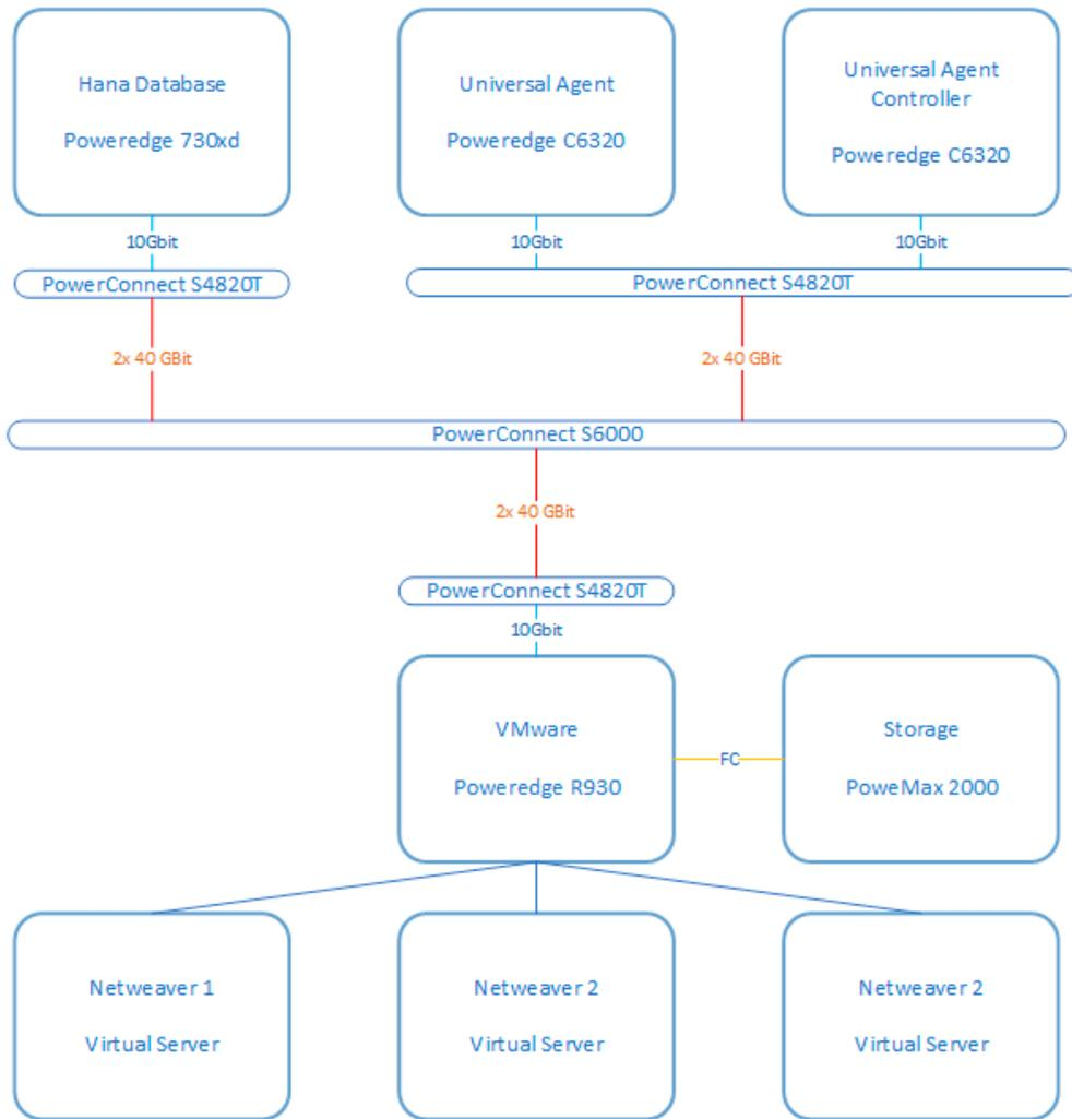
Figure 3: Dell hardware set-up
